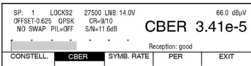
The bit error rate **before correction** (CBER), the bit error rate **after correction** (PER, packet error), the level, the carrier frequency offset, the modulation (QPSK or 8PSK) the code rate (CR), a possible spectrum inversion, the pilot signal (PIL) and the S/N value are displayed.
