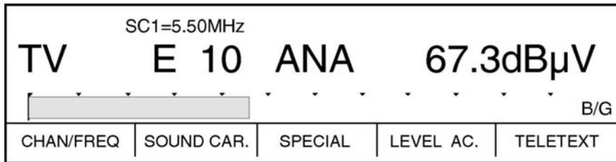
Use the **SPECIAL** key (F3) to call up menu in which the **TINT -** (F1) and **TINT +** (F4) keys appear. These keys allow you to adjust the phase (tint) in the NTSC colour standard. The phase setting is stored until the instrument is switched off.
