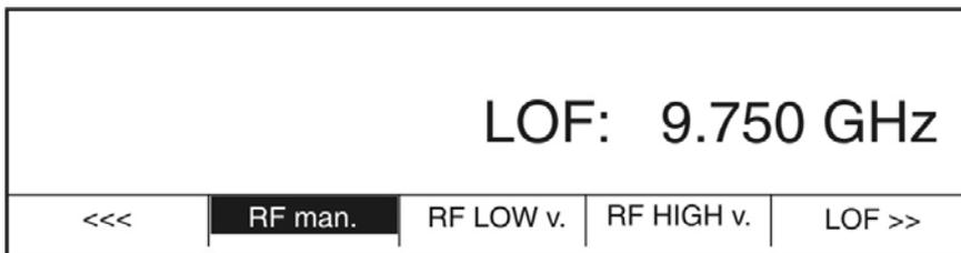
In variable mode, the 22kHz modulation switching criterion is **linked** to the use of the LNB local oscillator frequency and unlike with automatic mode, 22kHz modulation is not activated after the frequency that you have entered. Instead, frequencies are only accepted if they are possible with the previously selected 22kHz modulation (otherwise an error message is displayed, e.g. **FREQUENCY ERROR HIGH BAND IS SET**).
