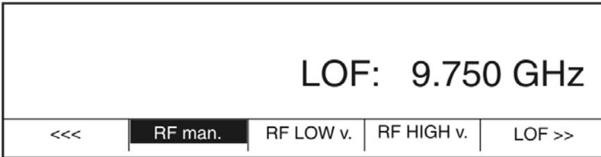
In this mode, the 22kHz modulation switching criterion is **not set** when the LNB local oscillator frequency is used.
