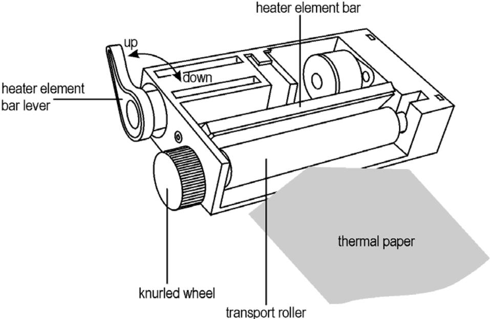
To feed in paper manually, raise the heater bar from the transport roller by pulling the lever up.
