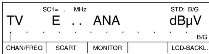
Enter a channel or frequency and then press **ENTER**. This sets the station, initiates the measurement and displays a TV picture.
