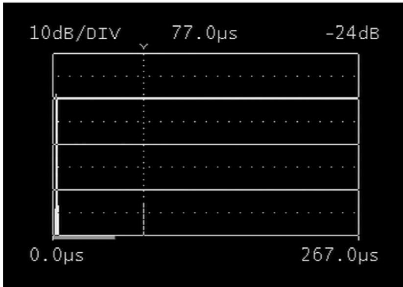
A primary impulse (primary reception direction) is shown on the left edge of the display. Additional smaller impulses can be seen to the right, in an interval with respect to time.
