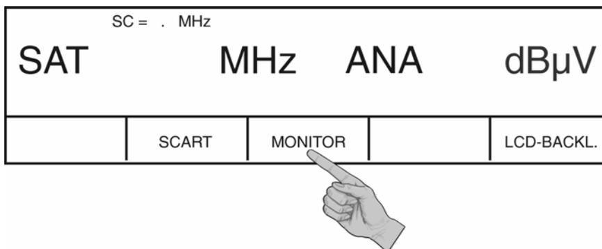
To do so, press **MONITOR** (F3) in the default mode of the instrument. The video signal fed to the scart socket is now displayed on the monitor.
