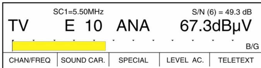
The figure in brackets after S/N indicate which line is being analysed. **Special program 89** allows you to select lines 5, 6 or 7.
