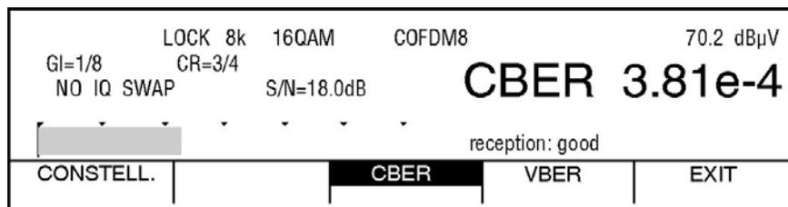
The bit error rate before Viterbi (CBER), the level, the guard interval, the code rate, possible spectrum inversion and the S/N value are displayed.
