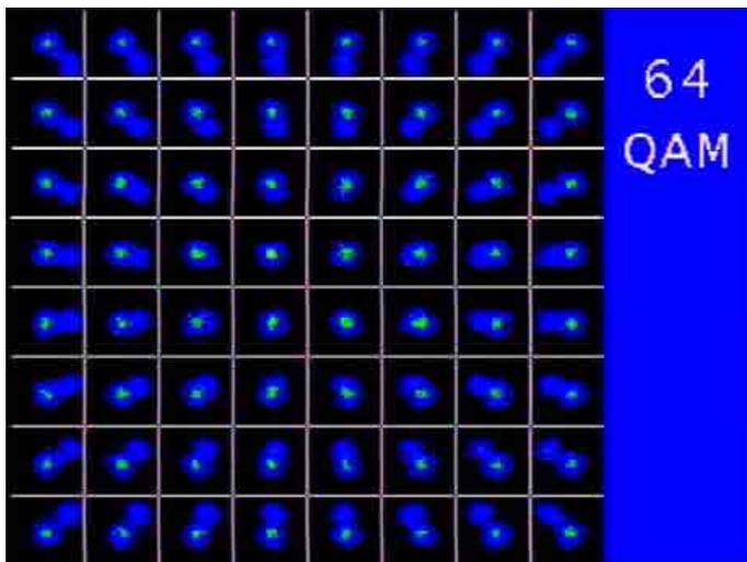
64QAM signal with IQ amplitude hum
