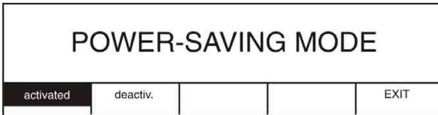
The currently selected setting is displayed inverted. The filter can be deactivated or reactivated using the F2 and F1 keys.
