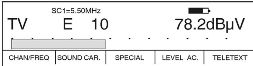
**Important!** ⚠ The dB indicator level (MODE 84) must be set to normal level; otherwise, the battery charge is not visible when measuring levels.
