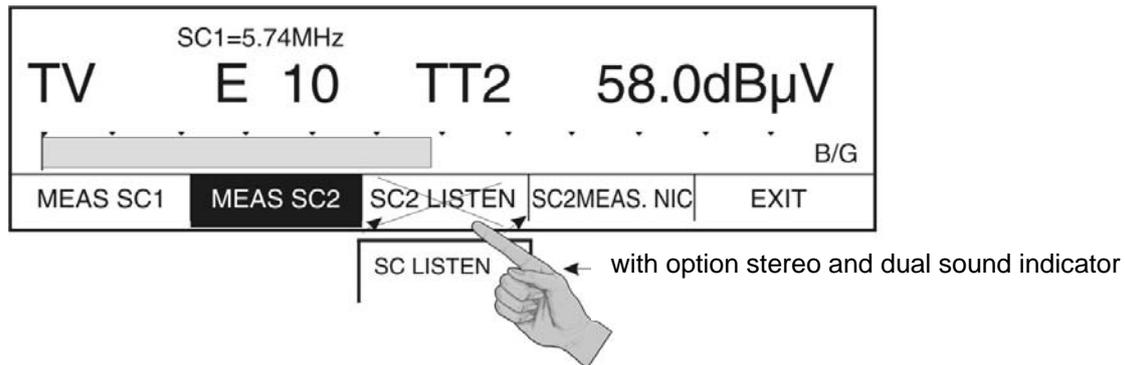
The **SC2** designation before the displayed level value indicates the selected measurement. Press the **MEAS SC2** function key (F2) again and the measured level of the video carrier is displayed.
