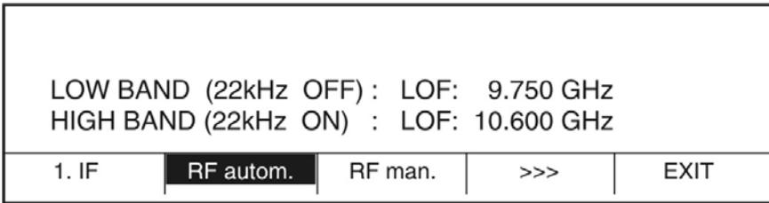
In this mode, the 22kHz modulation switching criterion is **permanently set** when the LNB local oscillator frequency is used.
