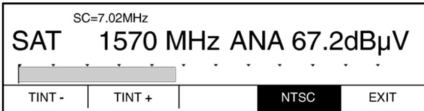
These keys allow you to adjust the phase (tint) in the NTSC colour standard. The phase setting is stored until the instrument is switched off.
