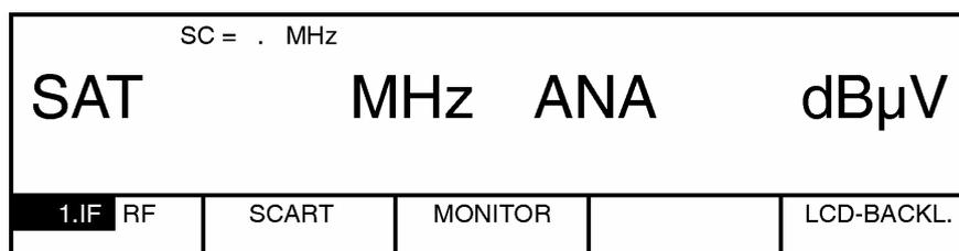
The display indicates that you must enter the 1st SAT-IF in MHz.
