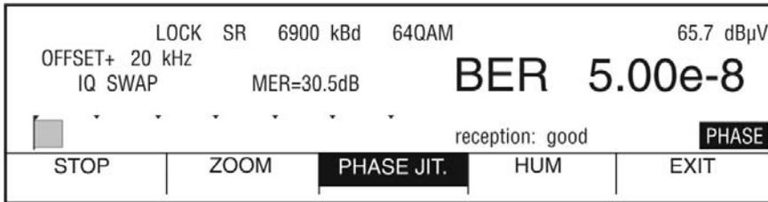
The **PHASE JIT.** (F3) function key is only visible when **ZOOM** is not activated.
