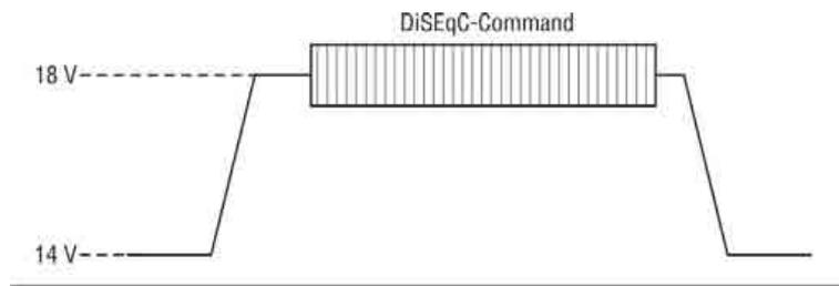
With UNICABLE systems, the transmitting receiver generates a high DC level as it transmits, to which is added to the UNICABLE message (special DiSEqC command). After transmitting the UNICABLE message, the receiver returns to an idle state, in which a low DC level is generated. The receiver must return to a low DC level, so that the system is available for other receivers.
