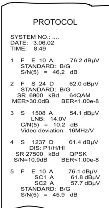
**Memory location 1:** TV range (F), channel E10, analog measurement (A), measured level, standard: B/G S/N measurement on line 5 (S/N(5)), S/N value (optional)
