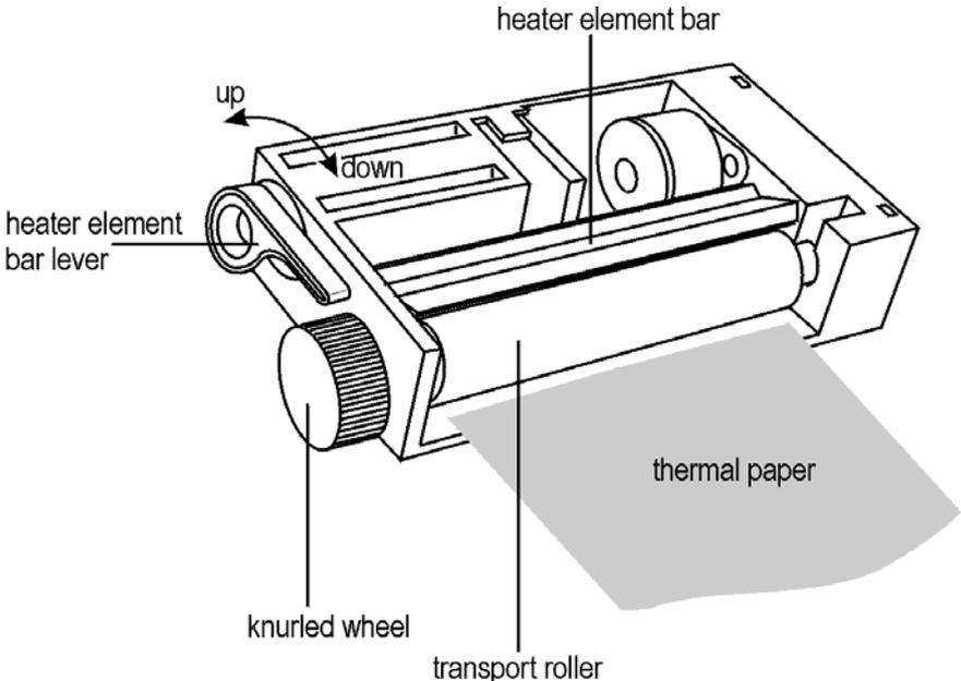
The instrument must be turned on and the heater bar must be on the transport roller (lever down).
