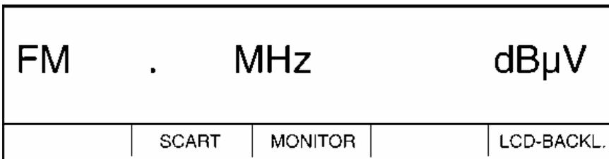
Enter the frequency with the numeric keypad. The spaces before and after the decimal point determine the number of digits you must enter.
