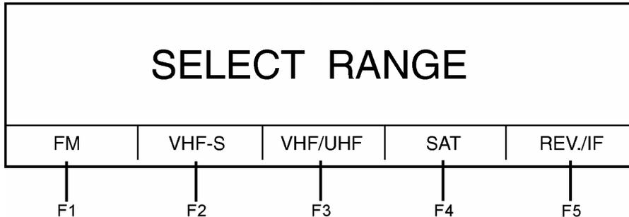
Use the function keys (F1-F5) to select a specific range. Digital measurements can be performed in the SAT (QPSK) range and the VHF-S or VHF/UHF (QAM, COFDM) range. Switch the instrument's mode to digital (DIG) with the ANA/DIG key.
