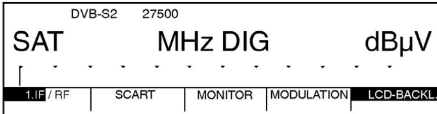
The standard set on the measuring receiver (DVB-S1 or DVB-S2) is displayed at the top left. Press the **MODULATION** function key (F4) to open a submenu which allows you to change the standard. The symbol rate can also be changed.
