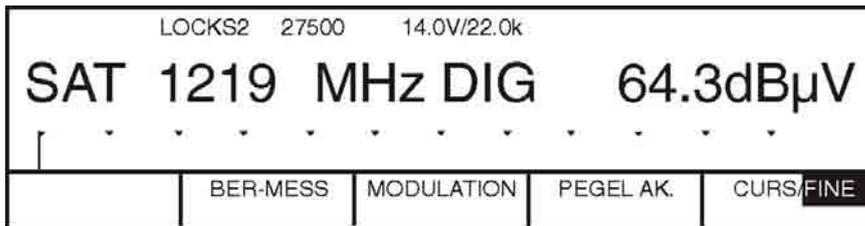
If the signal matches the standard set (DVB-S1 or DVB-S2), the device displays **LOCKS1** or **LOCKS2**; if not, **UNL-S1** or **UNL-S2** is displayed. If **UNL-S1** or **UNL-S2** is displayed, check the standard set and the symbol rate set.
