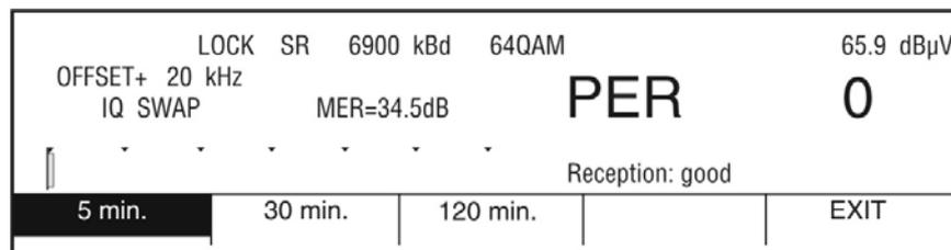
In this mode, the number of package errors is shown in the display. Package errors are added up until you leave this mode or the number reaches 60,000. The PER, MER, and level deviation are graphically recorded on the display.
