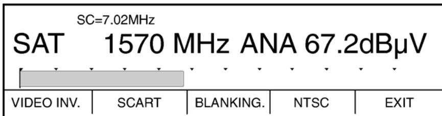
Use the **NTSC** key (F4) to switch to the NTSC colour standard in the SAT range. The **NTSC** function key is now displayed inverted. Two additional function keys, **TINT-** and **TINT+**, will appear at the same time.
