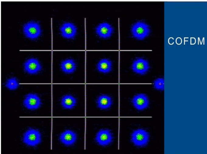
**Real COFDM signal with 16QAM**
