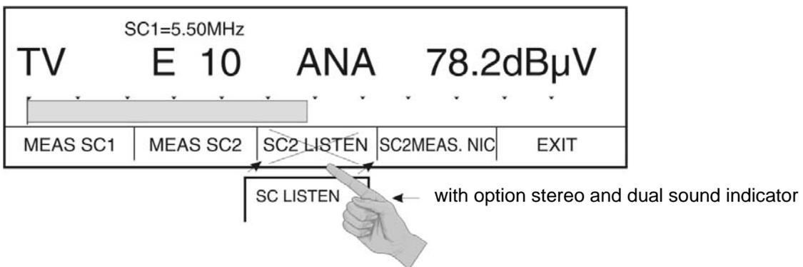
Selecting the **MEAS SC1** key (F1) displays the level of sound carrier 1. The **SC1** designation before the displayed level value indicates the selected measurement. Press the **MEAS SC1** key (F1) again and the picture returns and the measured level of the video carrier is displayed.
