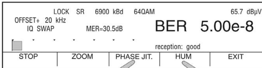
(only with instruments which 256QAM and Tuner TD1316) only with QAM
