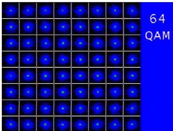
Poor signal-to-noise (S/N ratio)
