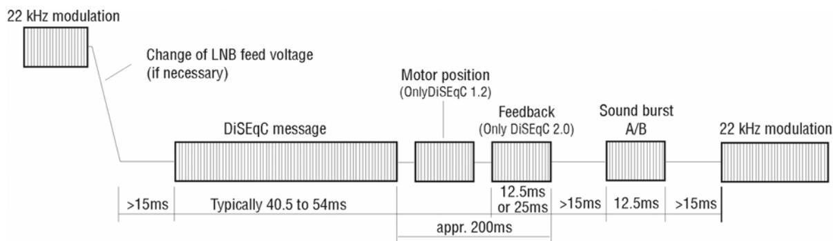
The 22kHz modulation, if present, is first switched off and the LNB supply voltage is set to the selected value. The DiSEqC message follows after a pause (The command for the motor position will be inserted for DiSEqC 1.2). With DiSEqC 2.0, a wait period of approx. 200ms is given for the return signal of the DiSEqC components. A sound burst is sent after about 20ms and, after an additional pause, the 22kHz modulation is switched on as well.
