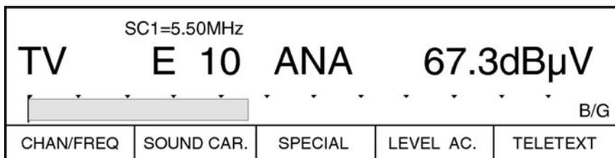
Press the **LEVEL AC.** key (F4) to activate the acoustic level trend indicator. The TV sound is switched off. The acoustic level trend signal can be changed using the volume control. The audio frequency of the level trend signal rises as the level increases and drops as the level decreases. This makes it possible to find the maximum of a received signal (eg, when locating an antenna).
