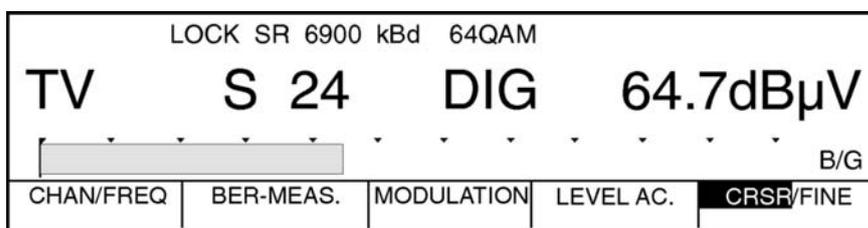
If a signal with the set modulation is present, the instrument responds with **LOCK** in the display; otherwise **UNLOCK** appears.
