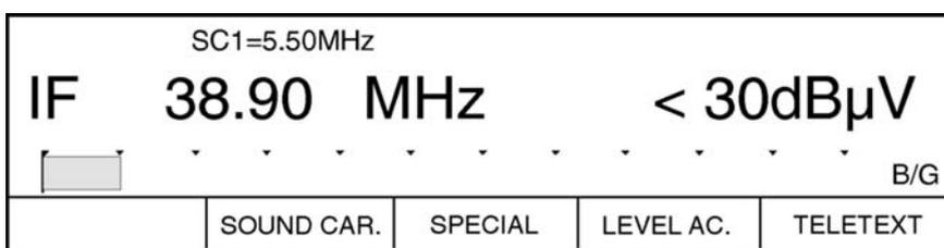
To display the teletext of the IF signal, press the **TELETEXT** key (F5). Refer to the **chapter on TELETEXT** for additional teletext functions.
