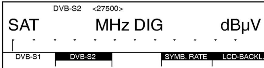
Then press the **SYMB. RATE** key (F4). The symbol rate in kSym/s (kBd) can now be entered via the numeric keypad. Press **ENTER** to save the changes.
