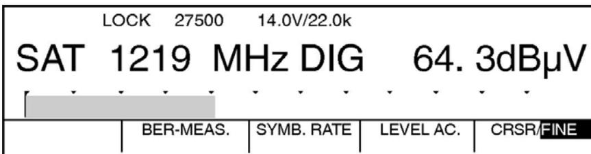
If a QPSK-modulated signal is present, the instrument responds with **LOCK** in the display, otherwise **UNLOCK** appears. If the instrument shows **UNLOCK**, the set symbol rate should be checked first. The symbol rate for the signal to be measured must be known and the set accordingly on the receiver.
