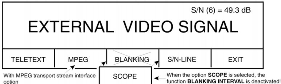
To display the teletext of the video signal, press **TELETEXT** (F1). Refer to the chapter on TELETEXT for additional teletext functions.
