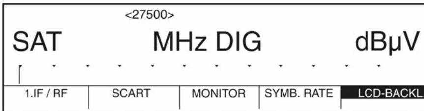
A frequency in the 1. SAT-IF range can now be entered. Press **ENTER** to initiate the measurement.
