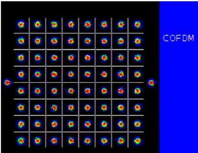
**Real COFDM signal with 64QAM**
