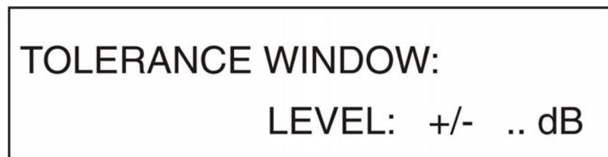
A value between 1 and 99dB can be entered using the numeric keypad. Press **ENTER** after you enter a tolerance level.
