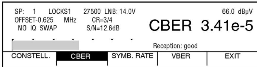
The bit error rate **before Viterbi** (CBER), the bit error rate before Reed-Solomon (VBER), the level, the carrier frequency offset, the code rate, a possible spectrum inversion and the S/N value are displayed.
