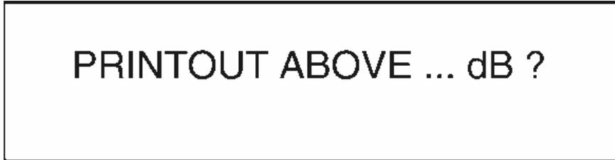
A new level can be entered using the numeric keypad. In the satellite range, this level may be between 40 and 119dBμV. In the remaining frequency ranges, the level may be between 30 and 119dBμV. Confirm the entry by pressing **ENTER**.
