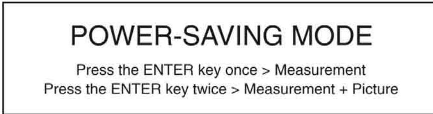
If the **ENTER** key is pressed, measurement can be carried out, but with a darkened screen. To reactivate the MPEG decoder and the screen, press the **ENTER** key again.
