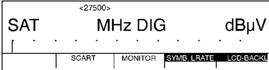
Press the **SYMBOLRATE** key (F4). The symbol rate in kSym/s (kBd) can now be entered via the numeric keypad. Press **ENTER** to confirm the entry.
