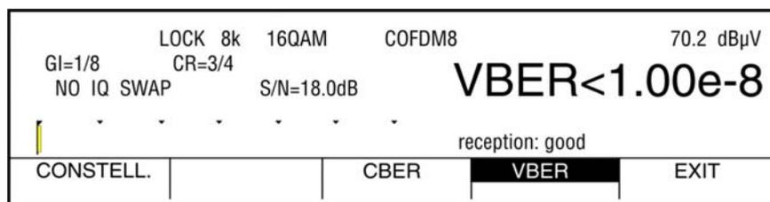
The error correction method implemented in the Reed-Solomon decoder is used to measure the VBER. Bit error rate measurement at this point in the receiver is identical for all three DVB reception modules (DVB-S, DVB-C and DVB-T).
