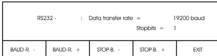
Now set the transfer rate and number of stop bits using the relevant function keys. When switching on the meter these adjustments are set to 19200 baud and 1 stopbit. The PC software is also working with these parameters.
