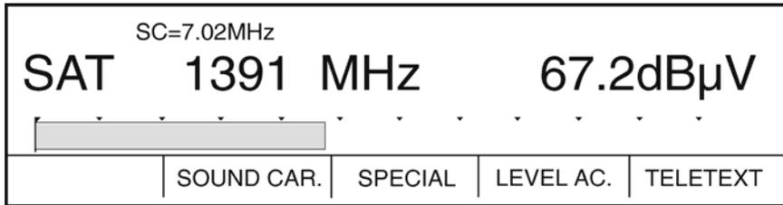
Press **SOUND CAR.** (F2) to access the sound carrier menu. The menu bar changes and the display appears as follows.
