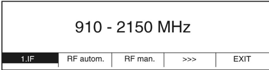
Use the function keys to select **1. SAT-ZF**, **RF automatic** or **RF manual** or other menu options. The selected operating model is displayed inverted.
