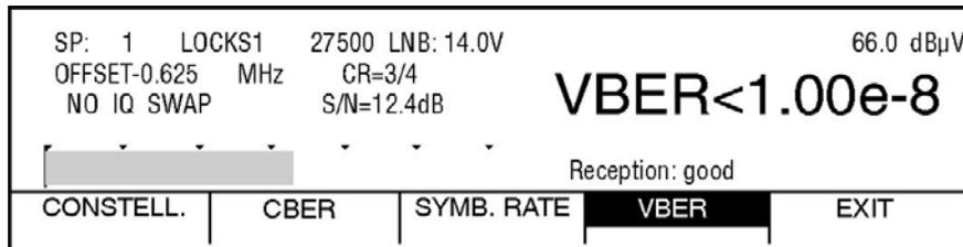
The error correction method implemented in the Reed-Solomon decoder is used to measure the VBER. At this point, the bit error rate can be measured in the receiver with all 3 DVB reception modules (DVB-S, DVB-C and DVB-T) in the same way. The following conclusion can therefore be made for all three reception types.
